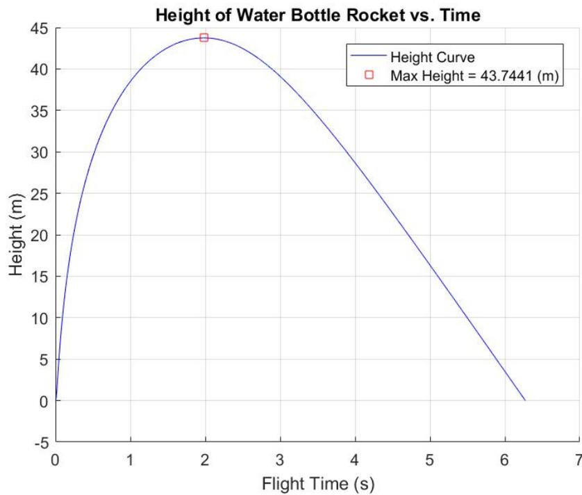
**Fig. 4.** Initial computational model of altitude over time of a water bottle rocket with: Volume of Bottle = 2 L, Launch Pressure = 60 PSI, Bottle Diameter = 0.110 m, (Volume of Water)/(Volume of Bottle) = 33%, Coefficient of Drag = .75, Empty Mass of Rocket = .074 kg
