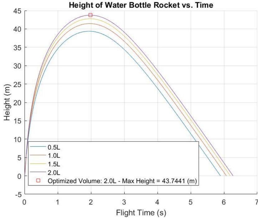
**Fig. 6.** Exploring optimal bottle volume using computational model of altitude over time of a water bottle rocket with: (Volume of Water)/(Volume of Bottle) = 33%, Launch Pressure = 60 PSI, Bottle Diameter = 0.110 m, Coefficient of Drag = .75, Empty Mass of Rocket = .074 kg
