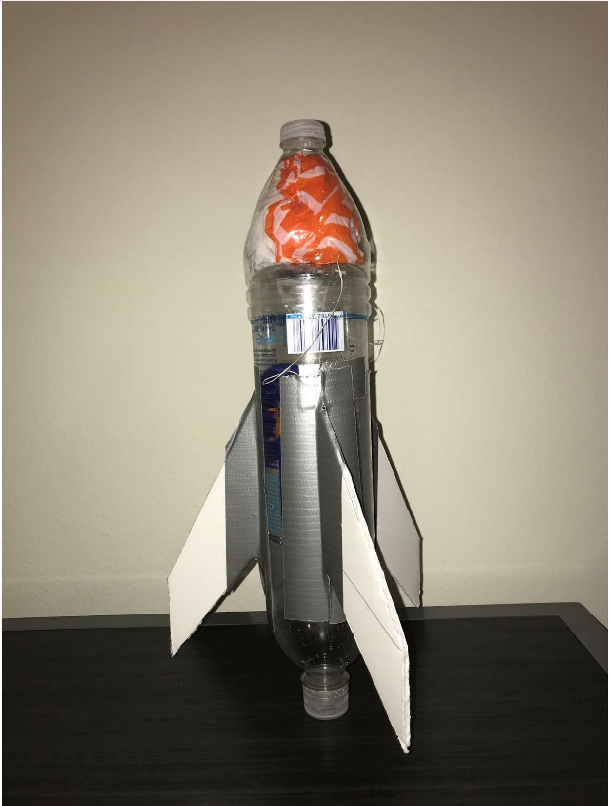
**Fig. 1.** Final Water Bottle Rocket Design
