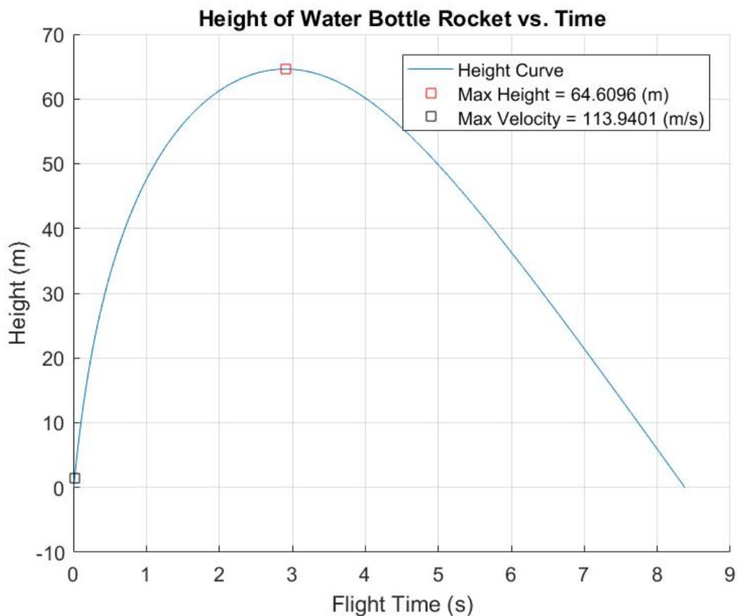
**Fig. 9.** Final computer model for height over time of final water bottle rocket with: Volume of Bottle = 1 L, Launch Pressure = 60 PSI, Bottle Diameter = 0.072 m, (Volume of Water)/(Volume of Bottle) = 4%, Coefficient of Drag = .75, Empty Mass of Rocket = .074 kg, using a correction factor of .8 for both height and velocity
