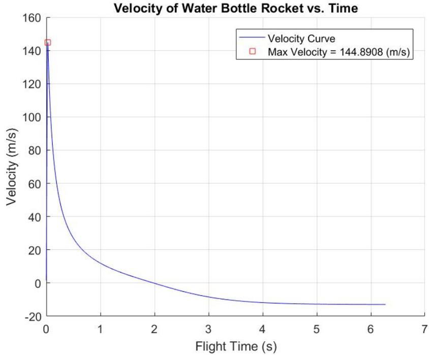
**Fig. 3.** Initial computational model of velocity over time of a water bottle rocket with: Volume of Bottle = 2 L, Launch Pressure = 60 PSI, Bottle Diameter = 0.110 m, (Volume of Water)/(Volume of Bottle) = 33%, Coefficient of Drag = .75, Empty Mass of Rocket = .074 kg
