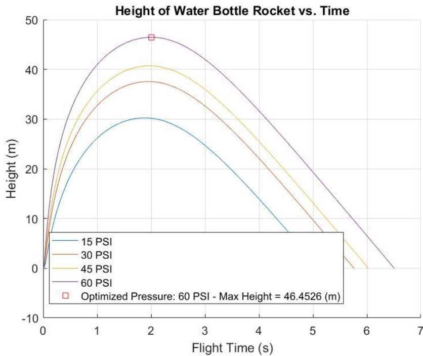
**Fig. 7.** Exploring optimal launch pressure using computational model of altitude over time of a water bottle rocket with: Volume of Bottle = 2 L, (Volume of Water)/(Volume of Bottle) = 33%, Bottle Diameter = 0.110 m, Coefficient of Drag = .75, Empty Mass of Rocket = .074 kg
