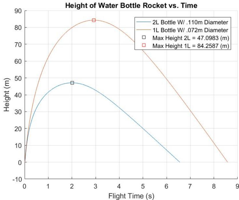
**Fig. 8.** Comparison of attitude over time of possible bottle volume/diameter combos of a water bottle rocket with: (Volume of Water/(Volume of Bottle) = 40%, Coefficient of Drag = .75, Empty Mass of Rocket = .074 kg
