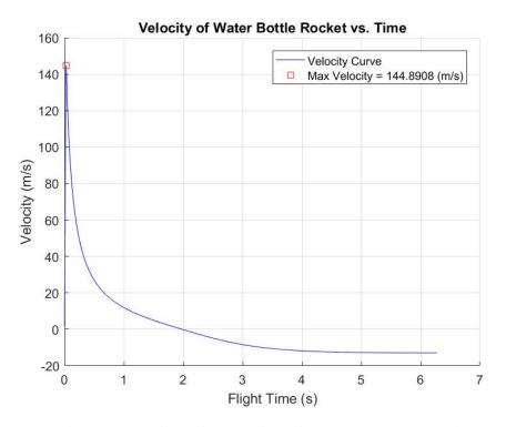
**Fig. 3.** Initial computational model of velocity over time of a water bottle rocket with: Volume of Bottle = 2 L, Launch Pressure = 60 PSI, Bottle Diameter = 0.110 m, (Volume of Water)/(Volume of Bottle) = 33%, Coefficient of Drag = .75, Empty Mass of Rocket = .074 kg
