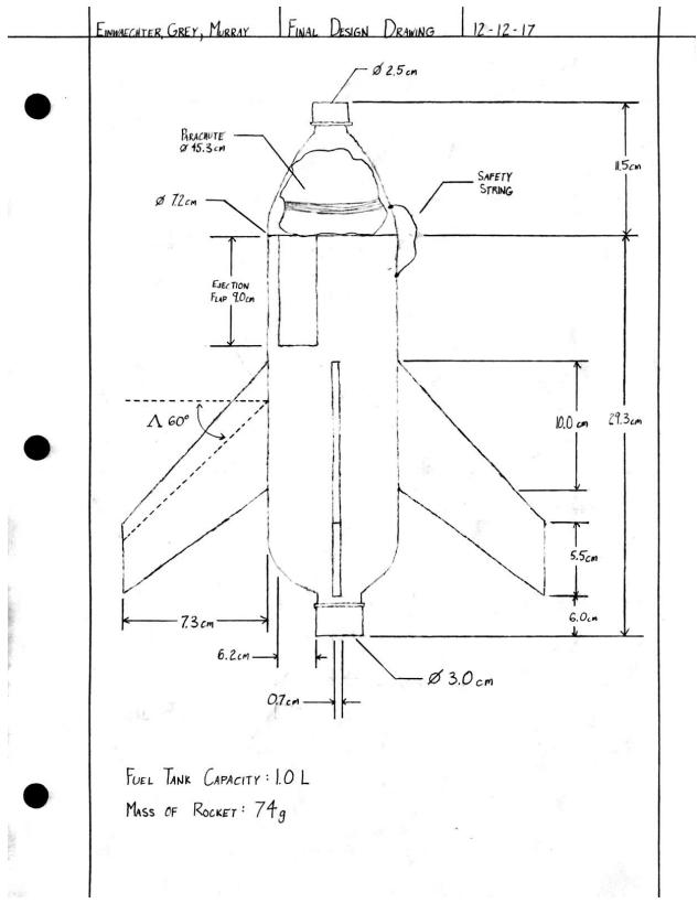
Fig. 2. Completed Dimensioned Drawing of Final Design
