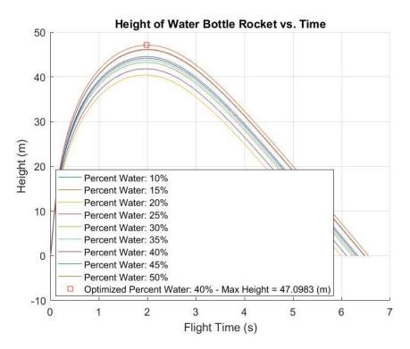
**Fig. 5.** Exploring optimal percent water, (Volume of Water)/(Volume of Bottle), using computational model of altitude over time of a water bottle rocket with: Volume of Bottle = 2 L, Launch Pressure = 60 PSI, Bottle Diameter = 0.110 m, Coefficient of Drag = .75, Empty Mass of Rocket = .074 kg
