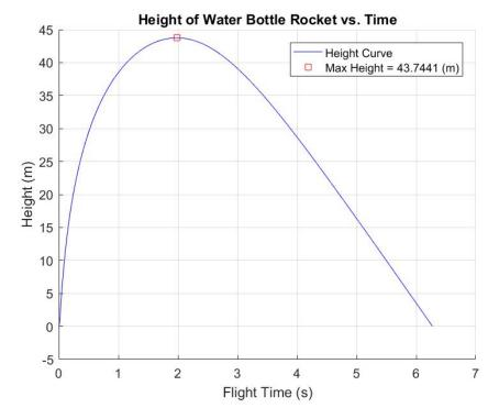
**Fig. 4.** Initial computational model of altitude over time of a water bottle rocket with: Volume of Bottle = 2 L, Launch Pressure = 60 PSI, Bottle Diameter = 0.110 m, (Volume of Water)/(Volume of Bottle) = 33%, Coefficient of Drag = .75, Empty Mass of Rocket = .074 kg
