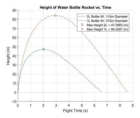
**Fig. 8.** Comparison of attitude over time of possible bottle volume/diameter combos of a water bottle rocket with: (Volume of Water/(Volume of Bottle) = 40%, Coefficient of Drag = .75, Empty Mass of Rocket = .074 kg
